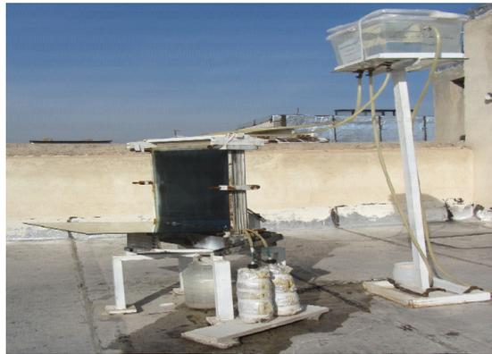
Fig. (2): Double-effect vertical diffusion solar still built in this study.
