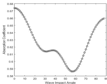
**Fig. (7): Absorption coefficient versus wave impact angle**
