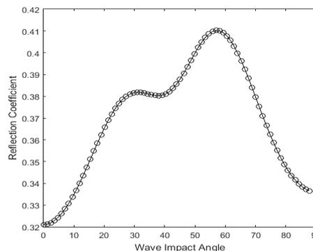
**Fig. (8): Reflection coefficient versus wave impact angle**
