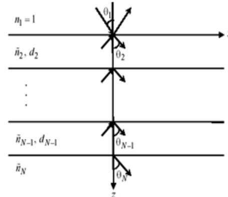
Fig. (2): The geometry for calculating the radiative properties of a multilayer structure [13]
