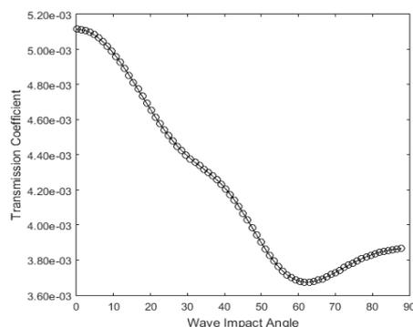
**Fig. (9): Transmit ion coefficient versus wave impact angle**
