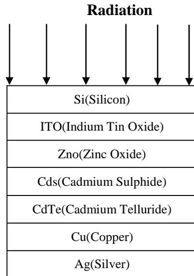
Fig. (1): Cross-section of a typical Cdte/Cds solar cell.
