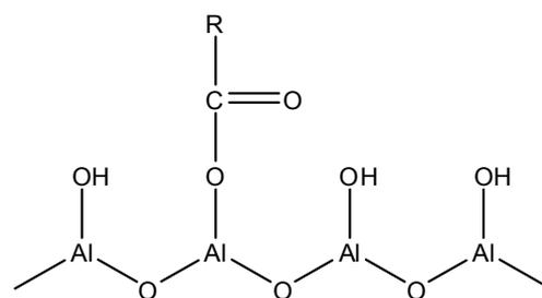
**Fig. (2): Molecular structure of Carboxylato-alumoxane**
