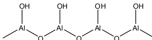
**Fig. (3): Molecular structure of Boehmite nano-particles**
