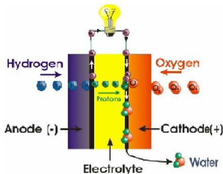
Fig 1. A schematic of a fuel cell
