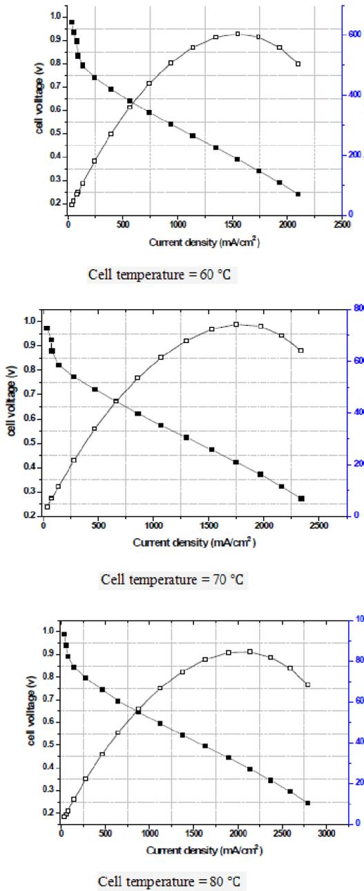
Fig4. The diagrams of voltage and output power changes in the fuel cell at pressure 15 psi (the relative humidity equaled 40 % in cathode and 100 % in anode.
