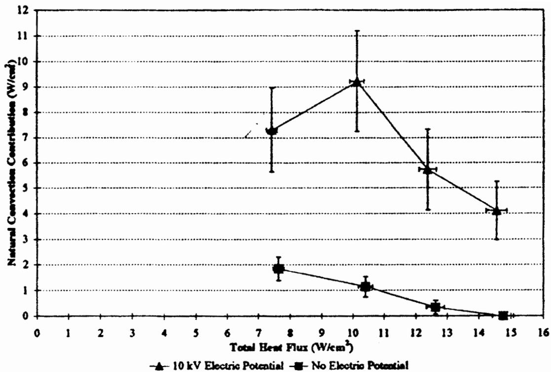
Fig. (1): (a) Relative heat flux contributions for experiments with no electric field. (b) Relative heat flux contributions for experiments with 10 kV electric potential ([3]).
