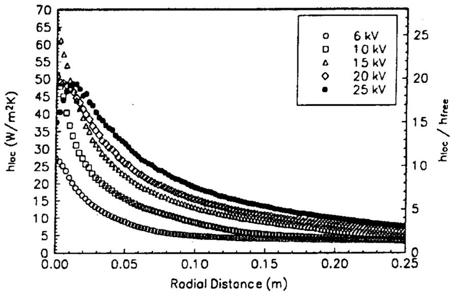
Fig. (3): Local heat transfer coefficients with various voltages and needle height of 5 cm ([20]).
