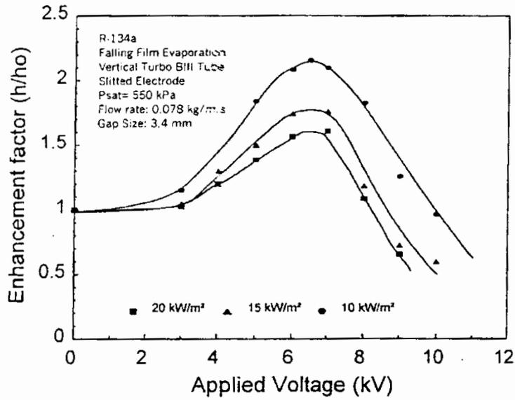
Fig. (2): Enhancement factor versus applied voltage on a Turbo Bill tube and a silted electrode ([11]).
