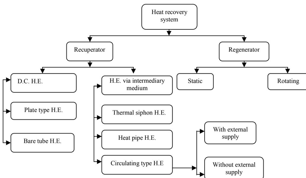
**Fig. (1): Classification of heat recovery system**
