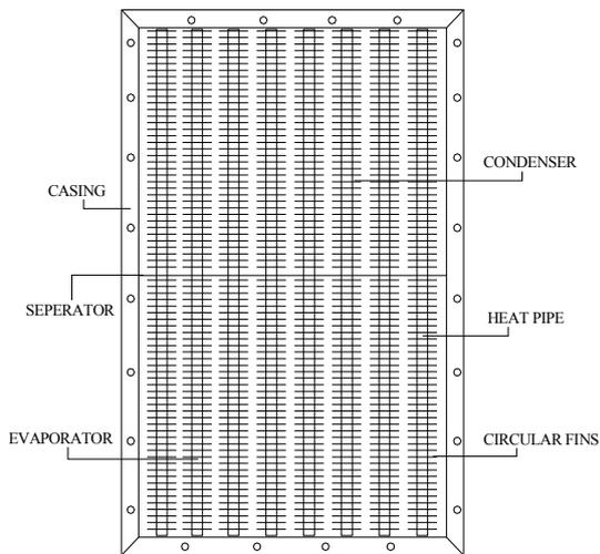
Fig. (3): Heat pipe heat exchanger
