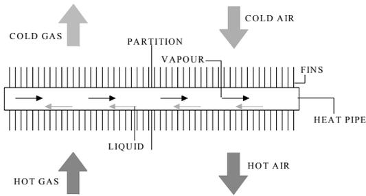
Fig. (2): Layout of a heat pipe.
