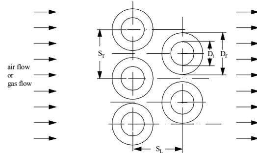
**Fig.(8):** Arrangement of heat pipes in heat exchanger
